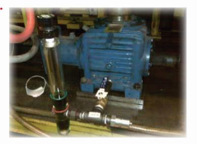
the gearbox drain ports to make oil drains easier. He suggested that the operator simply attach the hose from an existing filter cart to the quick connect whenever the oil needed to be drained, then use the cart as a convenient transfer unit to get rid of the used oil.
